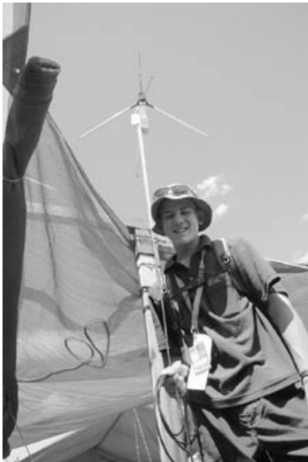
Photo 1 and 2 (above and above right): Nathaniel with his homebrew quarter-wave vertical for the 2-metre band.
