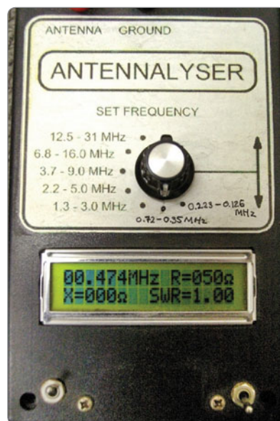
Photo 4: Additional switch positions on the front panel.
