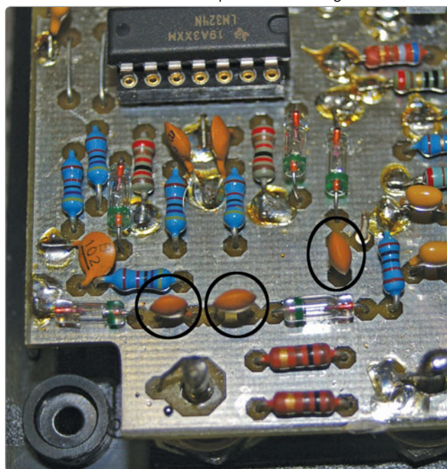
Photo 2: The three ceramic capacitors to change.
