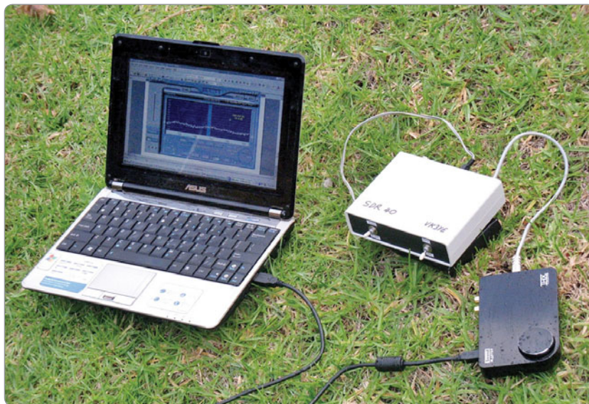
Photo 1: The receiver with the external Sound Blaster X-Fi Surround 5.1 Pro soundcard.
