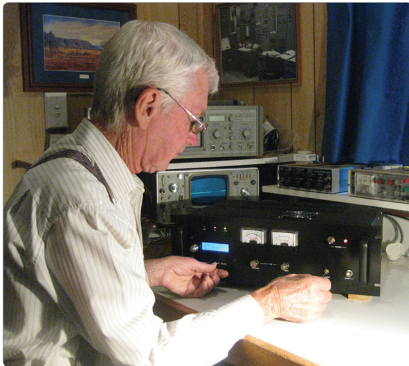
Noel VK3FI tuning the 630 metre transmitter.
