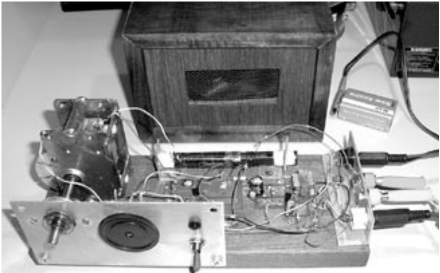
Photo 3: The completed regenerative receiver.
