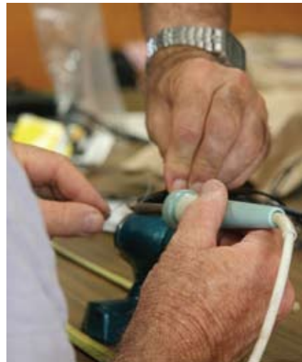
Soldering the stub to the half wave radiator
