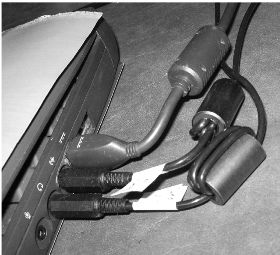
Figure 5: A view of the ferrite chokes and external PC screening.
