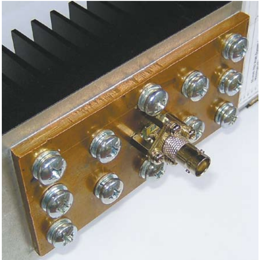
Photo 2: A close up view of the copper flange
