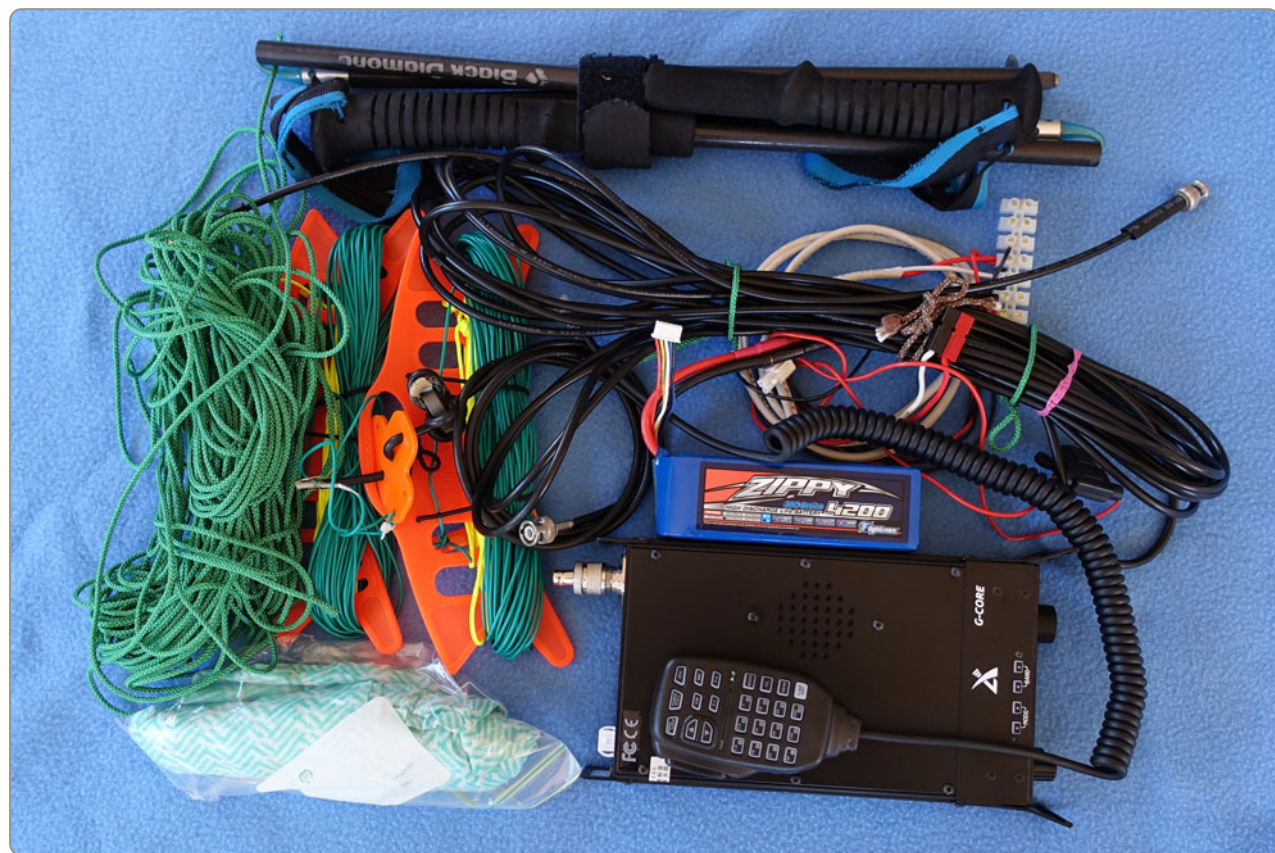
Equipment ready to pack for a Summits on the Air (SOTA) and Parks on the Air (POTA) trip with transceiver and leads, battery, cord to secure masts and/or hang a dipole from a tree, pegs, walking poles and dipole antenna. Not shown is a 7 m fibreglass telescopic mast.
