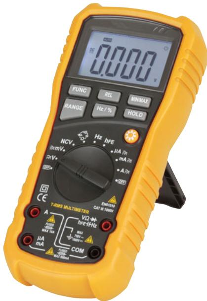
The **Digitech QM1321** is a robust, auto-ranging DMM with true-RMS AC measurement at an unpretentious price.
