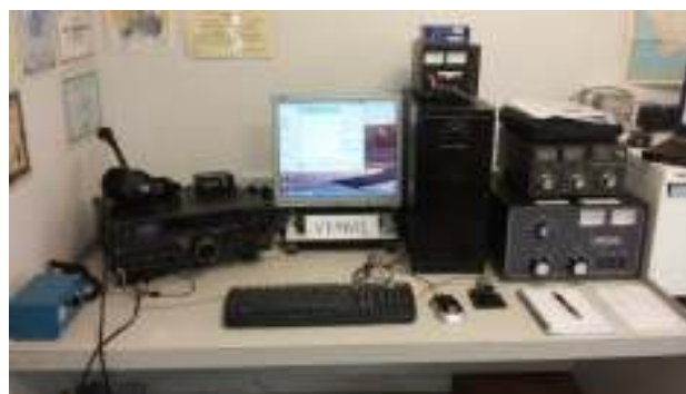
Figure 1 VK4WIL 14 & 3.5Mhz position. The big black box contains switchable coax stubs for 160-10m.
