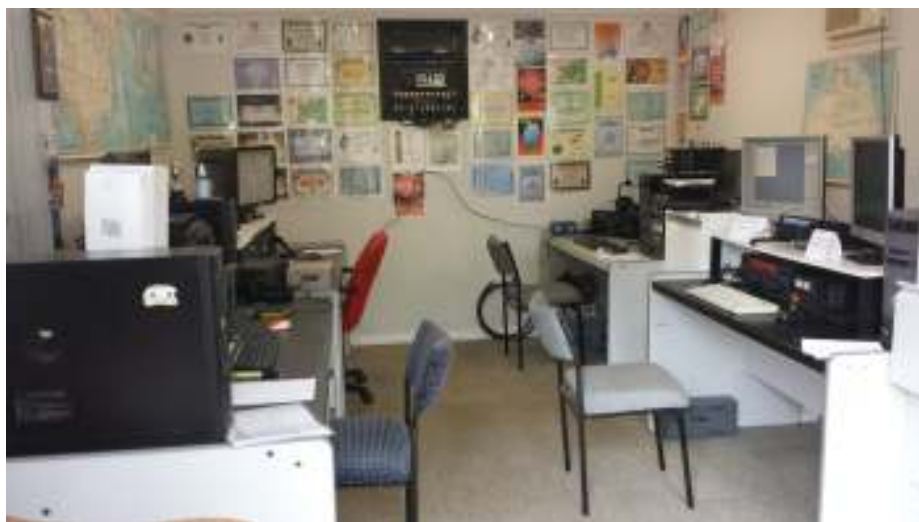
VK4WIL Multi-Multi shack made up for 4 positions. A mixture of coax stubs and band pass filters allowed operation on all bands without interference to one another.
